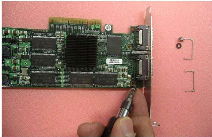
Figure 17: Attach Bracket onto Card using Screws
