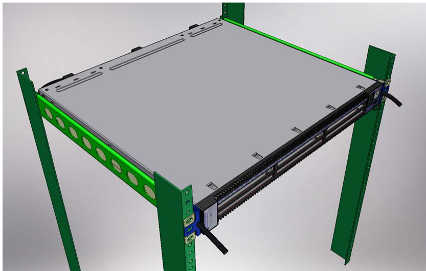
Figure 11: Transfer Power Cord Finished
