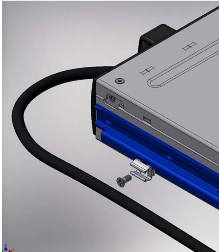
Figure 11: Install the Power Cord Clip
